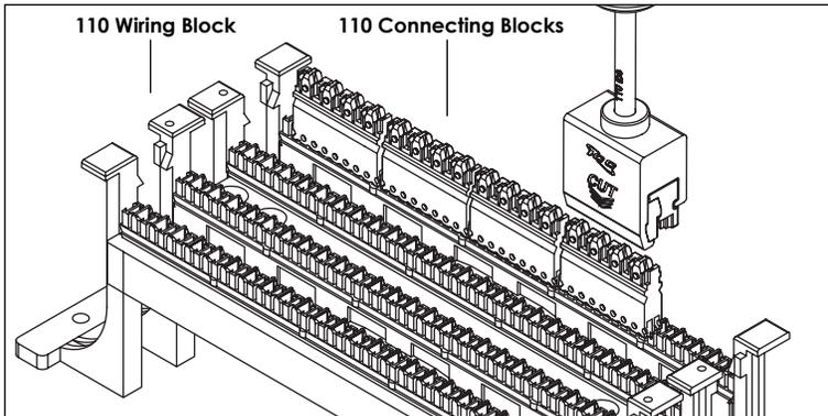
Step 1a: For seating 110 connecting blocks without cutting wire, use the tool as is. For terminating and cutting wire, follow the next set of directions.
