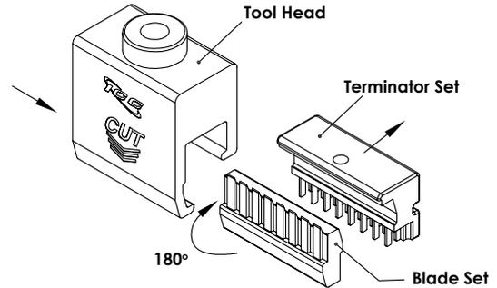
Step 1b: Push terminator and blade set out of tool head body from either side. Separate terminator set and blade set. Rotate blade set 180°. The blades will point down at this point.
