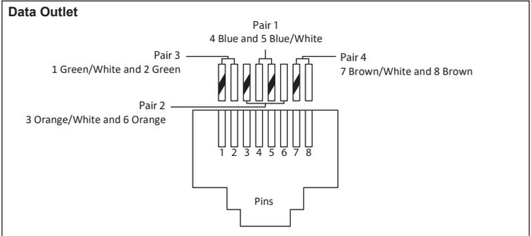
**Note:** It is important to follow T568A wiring because it allows pair 1 and 2 to be used for phone applications, up to 2 lines.
