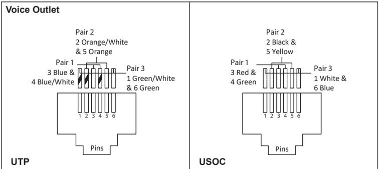
**Note:** Follow UTP or USOC wiring on 6P6C voice modular connectors to connect up to 3 phone lines per outlet.
