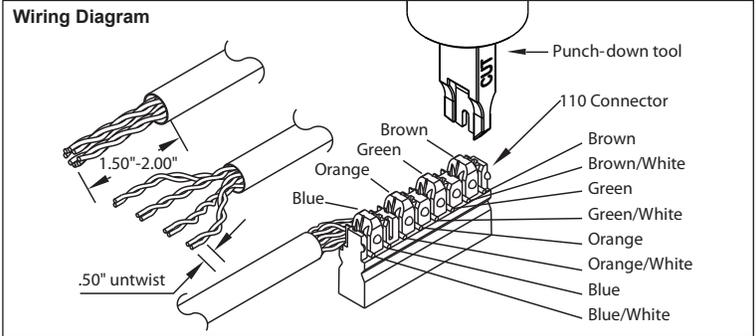
**Step 2:** Terminate the wires by only using a 110 punch-down tool. Be certain to follow the specified T568A color code for 8P8C installations as per TIA-570 residential wiring standards.
