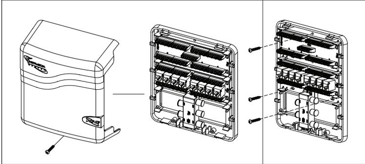
**Step 1:** Remove the screw to separate the cover from the base. Next, screw the base to a surface at a desirable indoor location using a minimum of 3 points.
