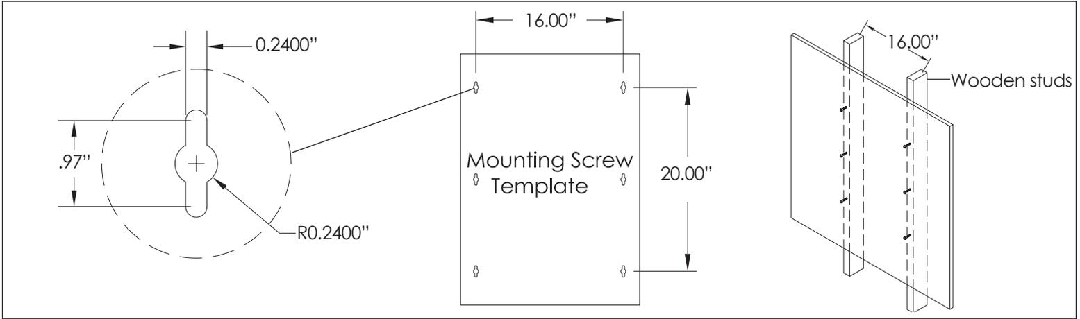
Step 1: Locate studs, then use the template to mark 6 locations for mounting screws (not provided). Pre-drill the screws without fully tightening them.
