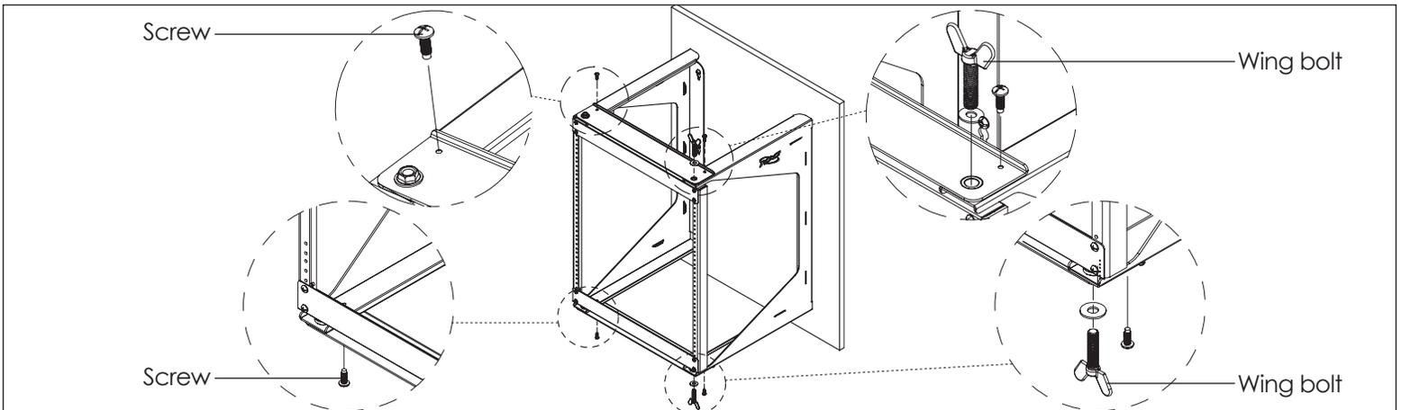
Step 3: Use four #12-24 screws and two wing bolts to secure the top and bottom of the frame to the brackets. **CAUTION!** Please do not exceed more than 85 lbs weight capacity.
