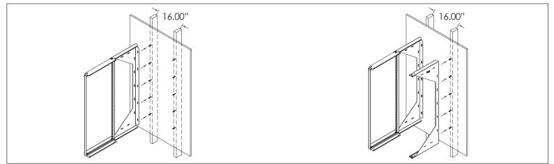
Step 2: Rack can be installed to swing open left or right. Place the left and right brackets onto the pre-drilled screws then tighten all screws.
