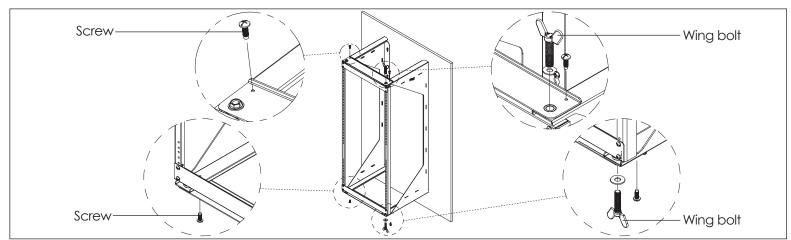
Step 3: Use four #12-24 screws and two wing bolts to secure the top and bottom of the frame to the brackets. **CAUTION!** Please do not exceed more than 85 lbs weight capacity.
