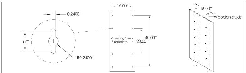
Step 1: Locate studs, then use the template to mark 10 locations for mounting screws (not provided). Pre-drill the screws without fully tighting them.
