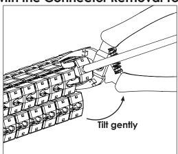
Step 1. Clamp the tool onto the connector. Step 2A. To remove connectors from the Step 2B. To remove connectors from the Note: Connector will break if tool is not placed top row, squeeze the tab and tilt the tool bottom row, squeeze the tab and tilt the gently and slightly upward.
