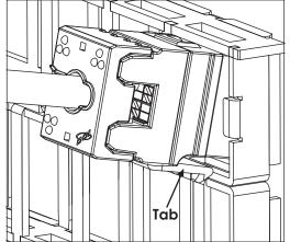
Step 2A. Insert the top row by tilting up 45 Step 2B. Insert the bottom row by tilting down The upper row of the connectors are installed degrees with the tab down.
