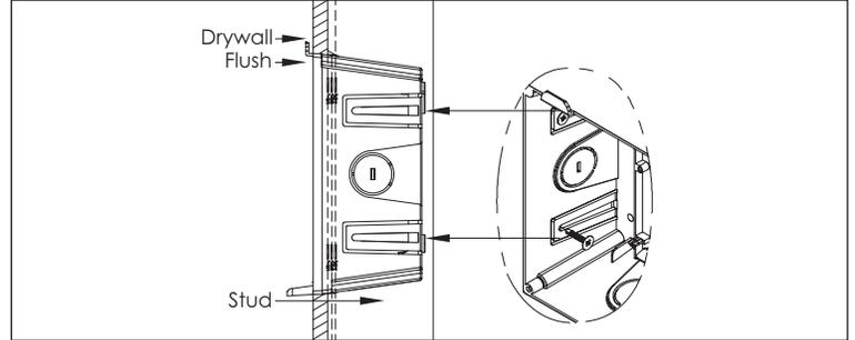
Step 2. Align the front of enclosure to be flush with the drywall or mounting surface. Once aligned, secure to the wall studs using the provided wood screws.
