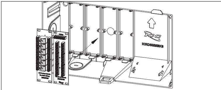
Step 3. Snap in the voice module in 1 of 4 available slots inside of the enclosure.
