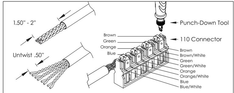
Step 4. To wire the telephone module, strip cable, place the wires into the IDC and terminate using a 110 punch-down tool. TIA-570 residential standard specifies T568A wiring. Note: One phone line per colored pair.
