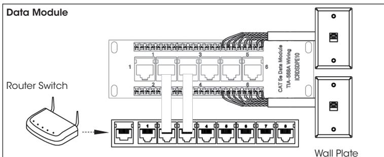
Step 6. Terminate cables on the 4-Pair 110 connectors on the data module. Connect one end of a patch cord to the corresponding jack and the other end to the Ethernet router after identifying the port to activate.
