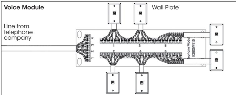
Step 5. Terminate the incoming phone line to the 110 IDC labeled "INPUT". Identify each outlet cable and terminate to 110 IDC labeled "1-6". Note: Line #1 = Blue; Line #2 = Orange; Line #3 = Green; Line #4 = Brown.
