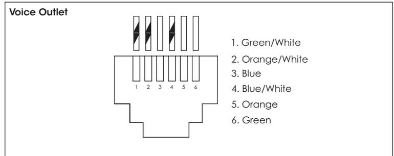
Note: Follow USOC wiring on 6P6C voice modular connectors to connect up to 3 phone lines per outlet.
