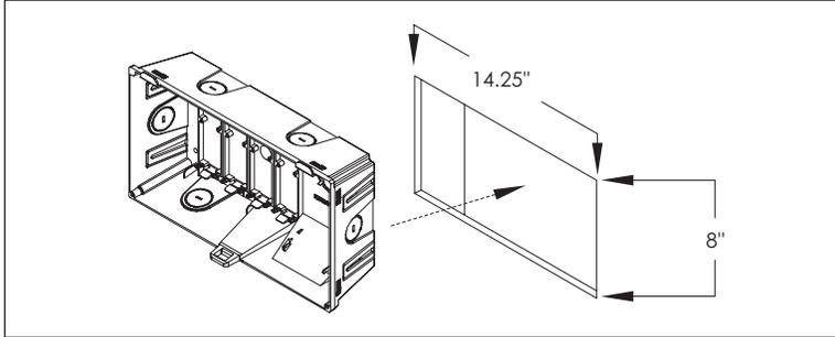
Step 1. Measure 14.25" width x 8" height and then cut an opening into the drywall. Place the enclosure into the opening.
