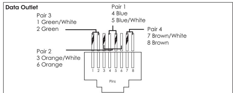
Note: It is important to follow T568A wiring because it allows pair 1 and 2 to be used for phone applications, up to 2 lines.
